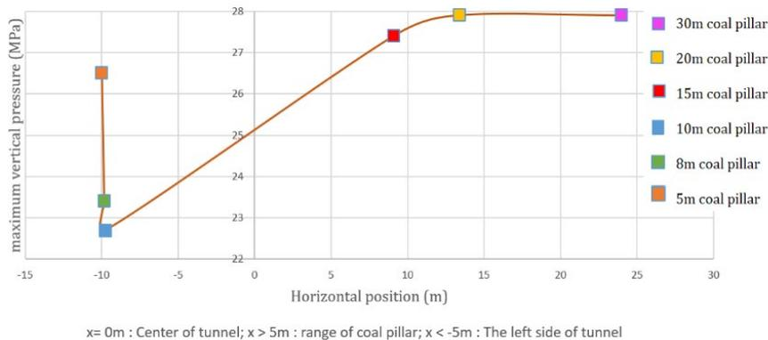
Figure 4. The maximum vertical stress on the top rock of vented tunnel No. 3.
