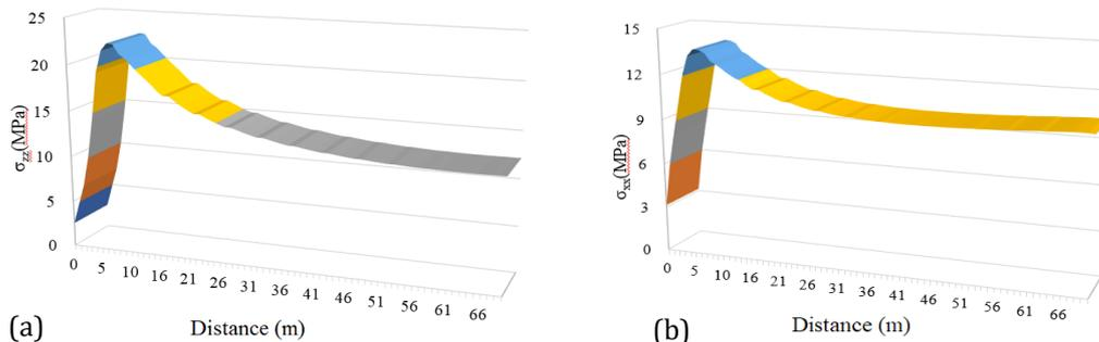
Figure 2. Stress distribution of the rock mass in the lower mining face LC2. a) vertical stress; b) horizontal stress.
