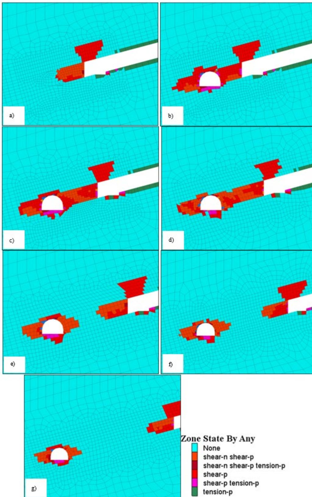
Figure 5. Distribution of the plastic destruction zone of the rock mass when the size of coal pillar changes: a - 0 m, b - 5 m, c - 8 m, d - 10 m, e - 15 m, f - 20 m, g - 20 m, h - 30 m.
