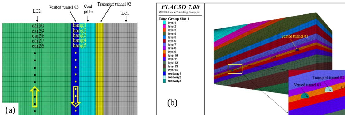
Figure 1. (a) The layout diagram of tunnels system; (b) Model on Flac3D.
