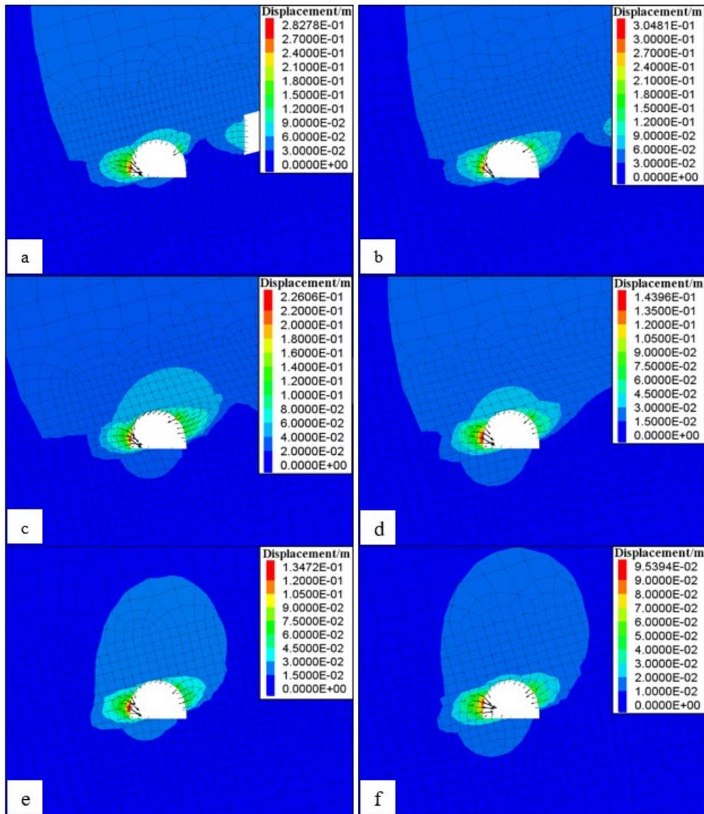
Figure 6. Rock mass displacement characteristics around the auxiliary tunnel No. 3 when the size of coal pillar changes: a - 5 m, b - 8 m, c - 10 m, d - 15 m, e - 20 m, f - 20 m, g - 30 m.
