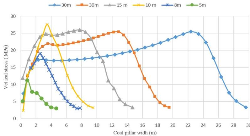
Figure 3. Vertical stress in the coal pillar.
